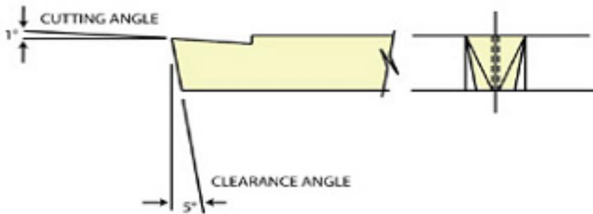
These are the grinding angles I use on my tools. Textbooks say that for brass the cutting angle should be nil, but I have about 1 degree and find that with this I can use the same tools for hardwood and for brass. After grinding I do give the tools a bit of a polish to the cutting faces on an India oil stone
