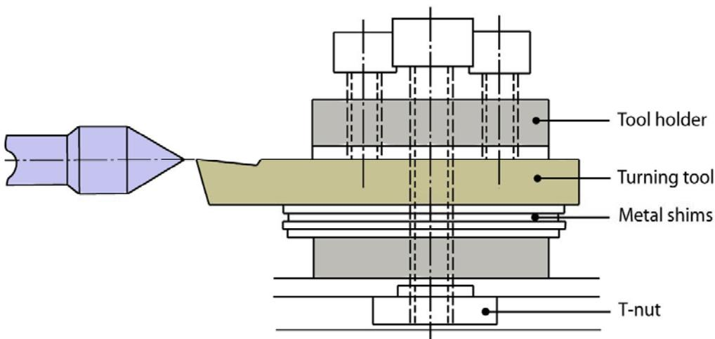
When turning small diameters it is essential to ensure the tool tip is exactly on the centre line of the work. Adjust this by adding or removing shims from below the tool.
