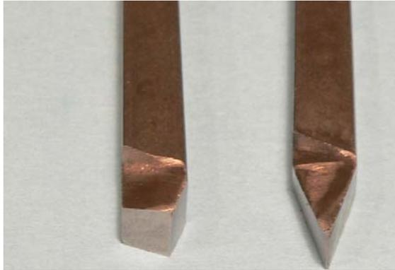
Shown here are the right hand planing or turning tool and the pointed turning tool. They are made from HSS steel.
