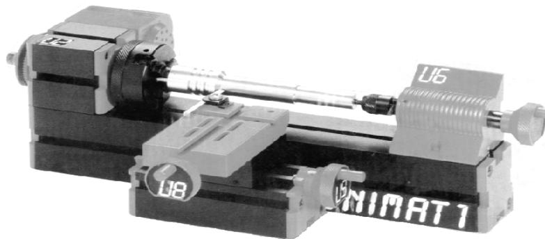
A strange animal this coming as it does from Unimat! The bed rail is thin aluminum, the optional chuck is white metal the rest is all plastic and it has a 12 volt motor. The best I have heard about it is that it is quite good at machining wax.
