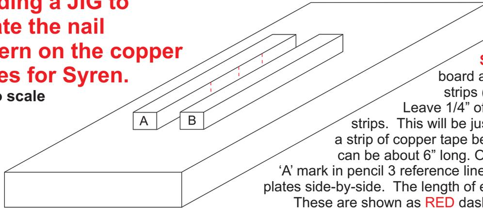
**Step One** - Take a scrap board and glue two  $\frac{3}{16}$ " x  $\frac{1}{4}$ " strips (A & B) down the center. Leave  $\frac{1}{4}$ " of space between the two strips. This will be just enough space to slide a strip of copper tape between them. The strips can be about 6" long. On the inside side of strip 'A' mark in pencil 3 reference lines to indicate two copper plates side-by-side. The length of each plate will be  $\frac{11}{16}$ ". These are shown as RED dashed lines in the drawing.
