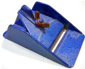
Loom a line; the general consensus is that this tool is useless. Despite having tried it a several times the result is always the same, give up in disgust. It is supposed to allow you to construct rat lines off the ship. It just that the finished product never seems to fit the ships. All in all it's an easier and better job to do the rat lines on the ship.
