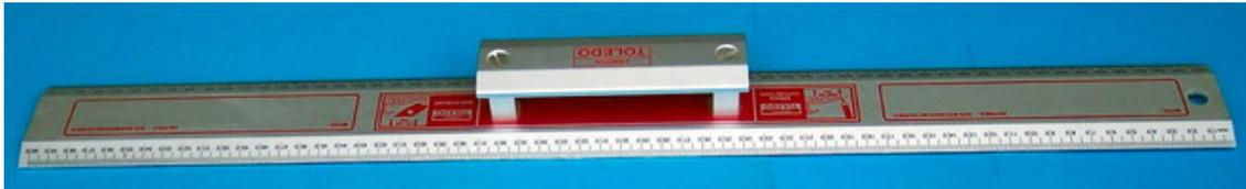
Razor saw and additional blades. It's a good idea to store the blades with the teeth imbedded in a piece of scrap balsa wood for protection.
