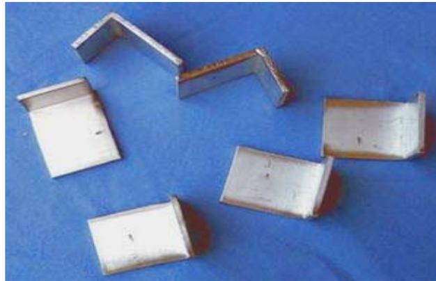
Machinists squares; a good way to ensure that the first bulkhead is absolutely true and if nothing else a good machinists square is needed to check that the angle of the aluminium squares is exactly 90 degrees.
