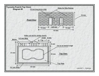
way that I made mine was to use .005 thick 36-gauge copper. Cut strips 42 mm long and at least 20 mm wide. These should go all the way to the floor base and still have about 21 mm sticking out the top. Wrap the copper around a strip of wood 1/8"x 3/16" (3x5 mm). Now this is not the best way to do this, but I glued this together with CA glue.
