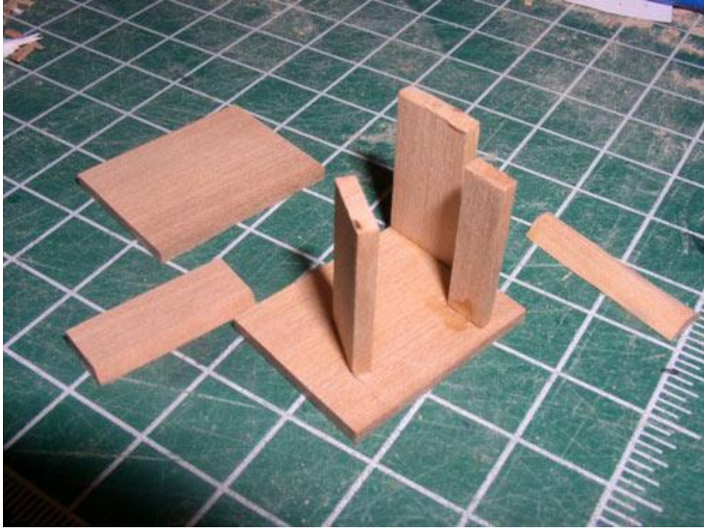
Photo 1 shows the pieces of the stove base. Some may chose to make this of metal, but I found it easier to use wood, boxwood in this case. These were glued together with ordinary aliphatic carpenter's glue.
