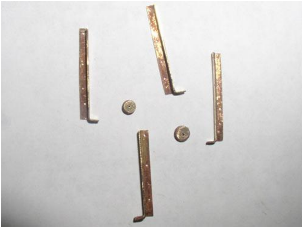
Photo 2 shows “iron” corner pieces that held the sidepieces together. Brass angle iron can be found in most any hobby shop. I had to grind and file these corner pieces, as both sides of the “L” were too large to be in scale. The ends of the corner bars need to be trimmed so you can bend and form feet. Note that there are two lefts and two rights. The pulleys in the photo have no business in this photo and will be explained later.
