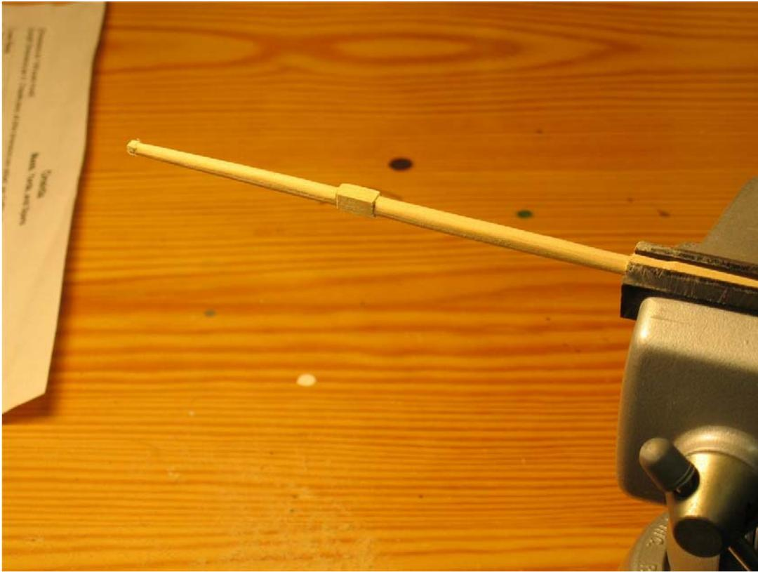
I now use a strip of 220 grit sand paper, my trusty hand drill, and begin to get a fine, smooth finish on the mast. If one happens to break the mast at this point it conveniently falls directly into the trash can, below.
