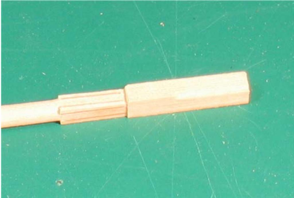
In this photo I've already filed the octagonal section near the heel and am working on the hounds. I first file the hounds to octagonal, but without the taper, and then come back and gently file the taper, working from the lower end up. This is the one portion of my process that takes some finesse.
