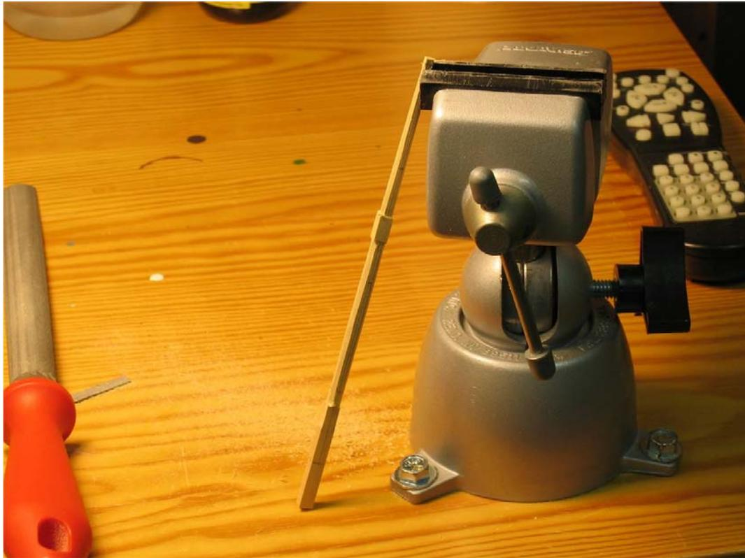
I now move on to using a fine, flat file. The next step is to turn that eight sided mast into a 16 sided mast. Since marking the lines would cause more errors for me than it's worth I just begin filing the edges of the eight sides. With little effort the mast becomes very close to a tapered circular section
