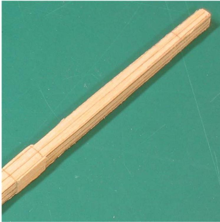
Back to the Dremel to sand the taper into the second sides of the mast, perpendicular to the first marked and sanded sides.
