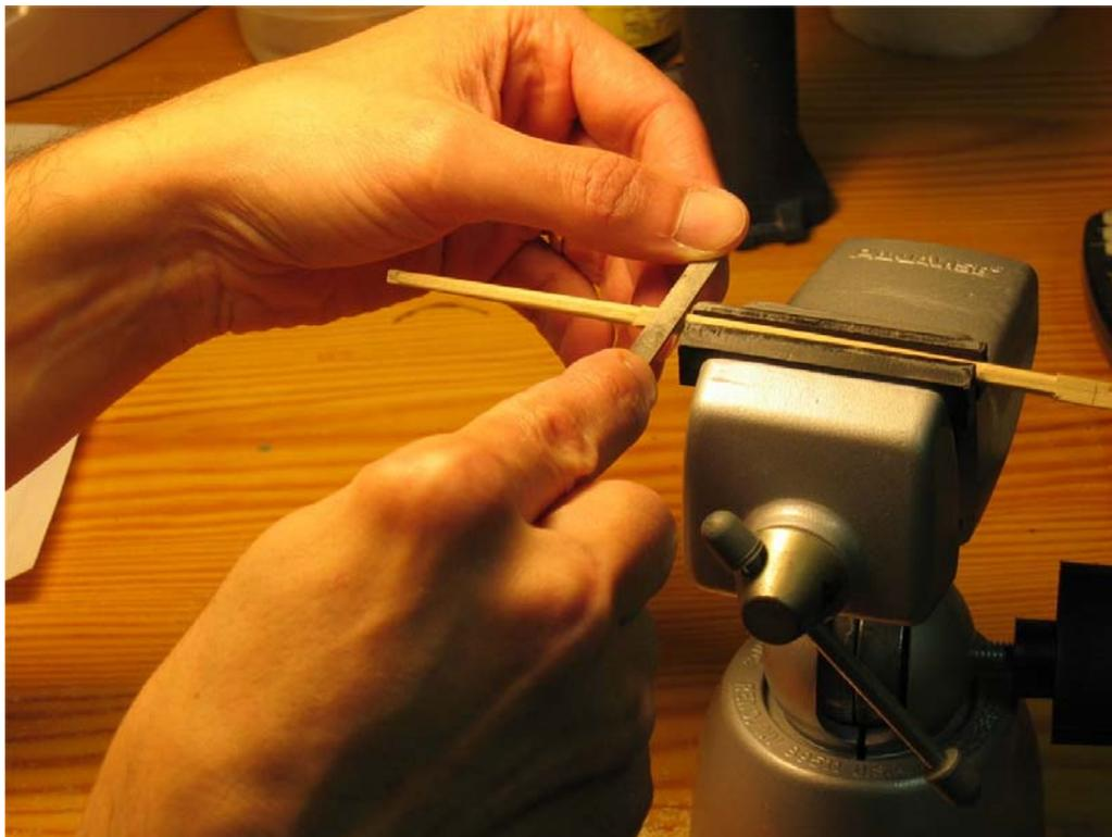
I'm now cleaning up the upper edge of the hounds with a chisel; the fine flat file works well for this, too.
