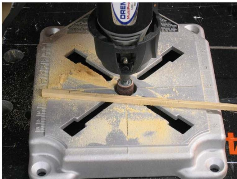
Back at the workbench you can see the two sanded sides. I've used a fine, flat file to clean up the edges at the hounds and the heel. I've now transferred the taper curves of the mast to the side adjacent to the first marked side.
