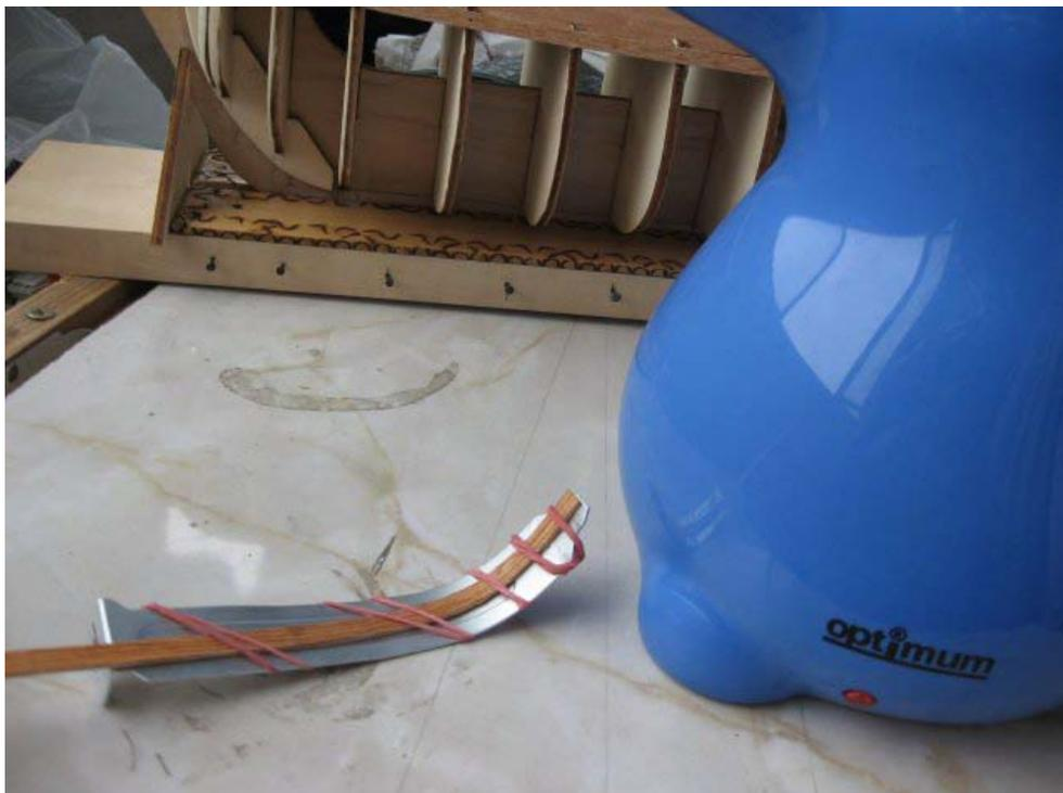
**Figure 4. – Planks Drying on the Shaped Metal.**
