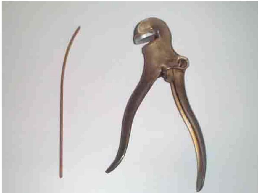
**Figure 2. – Plank Bender adapted from a Saw Set Device .**
