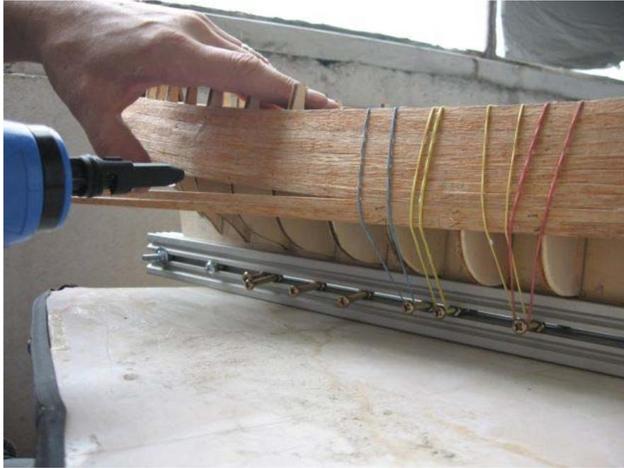
Figure 16. – Using the Steamer to Form planks on the Model.
