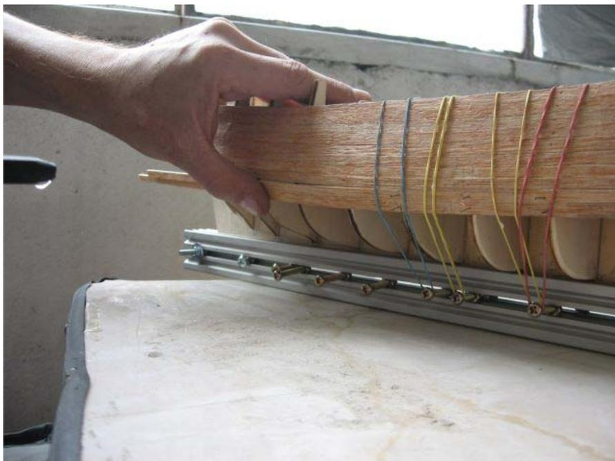
Figure 17. – The Formed Plank on the Model.
