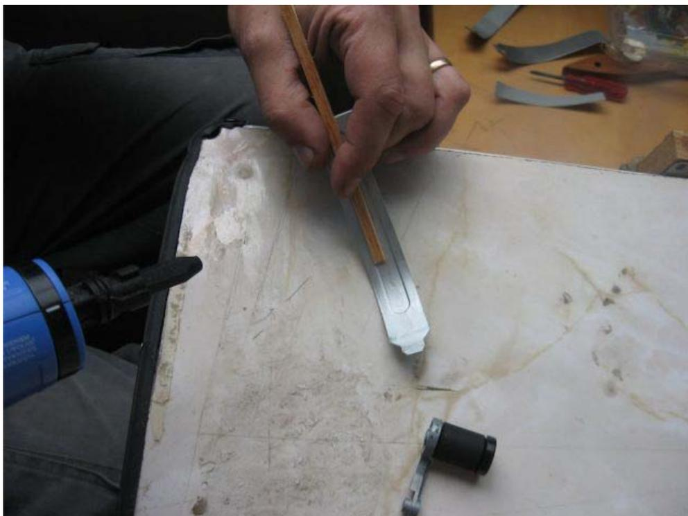
**Figure 11. – Continuing to Bend a Plank.**
