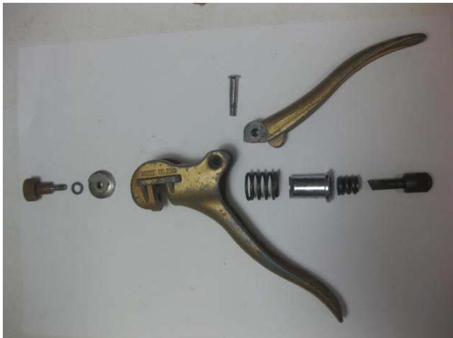
**Figure 4. – Exploded view of the Plank Bender.**
