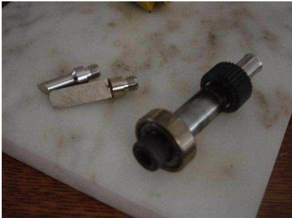
**Figure 2. – The New Tip with the Removable Old Tips.**
