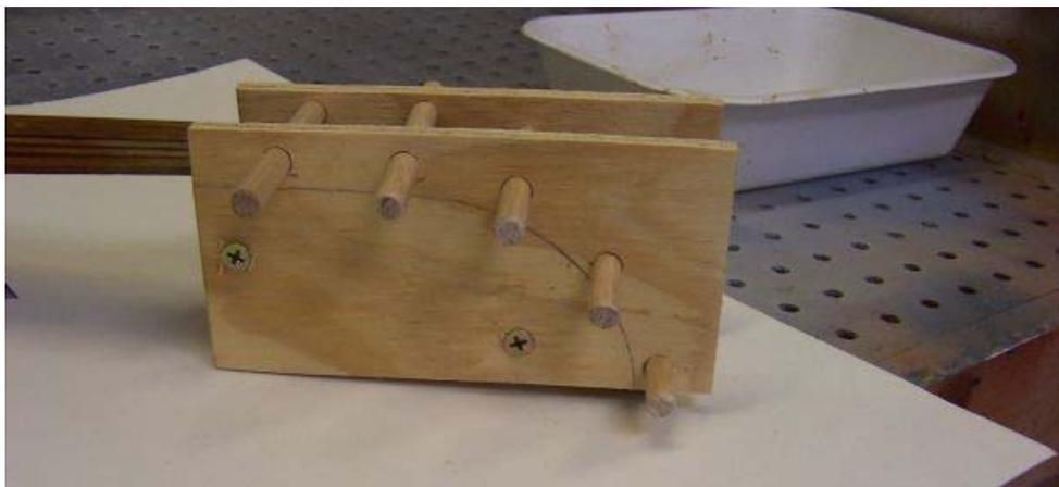
**Figure 2. – Bending Jig Detail (reklein)**
