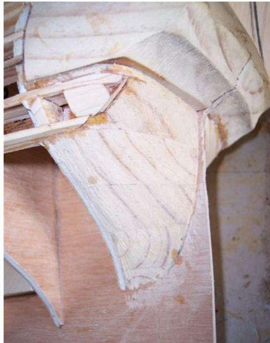
The transition of the lower part of the filler block to keel should be smooth flowing without bumps. The idea is to have the planks flow smoothly over the filler block at this point and onto the false keel. Of course the filler block changes shape as it rises and it may be that it eventually winds up at right angles to the keel as in my case. It all depends on the ship you are building, so follow your plans closely.
