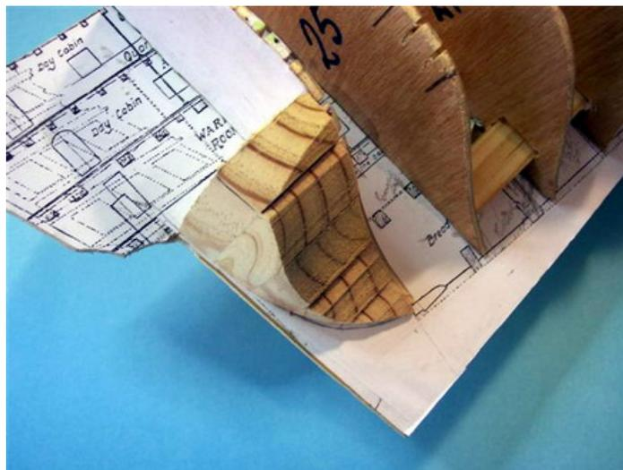
I used a sanding drum in a small drill press for this shaping but again this can be accomplished by hand sanding and or the use of files and carving chisels. Just go steady and carefully.
