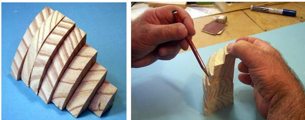
Next make up a paper card template from your plans of the keel. The bearding line will be the forward shape. When this template is placed on the keel side of the filler blocks this will establish the inside shape of the blocks.
