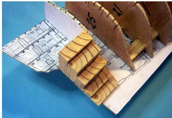
Now mark the outline of the last bulkhead onto the forward side of the filler block assembly. A template can be made up for this operation if you prefer.
