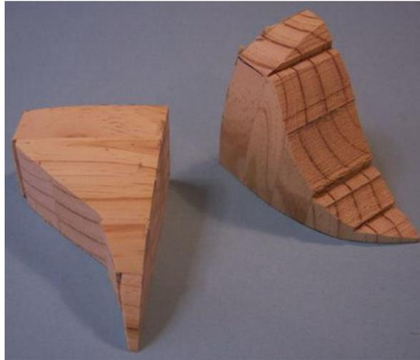
**IMPORTANT:** Make sure the shapes you are going to make are side for side and not as I have done in the past identical to each other so that I have two blocks for the one side instead of one for each side. An easily done thing so check and double check, don't assume.
