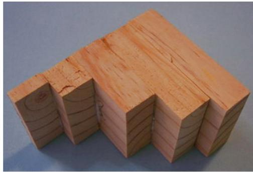
Glue the blocks together, when dried place them into position BUT DON'T GLUE them at this stage to the keel or bulkhead. This is only a marking out step.
