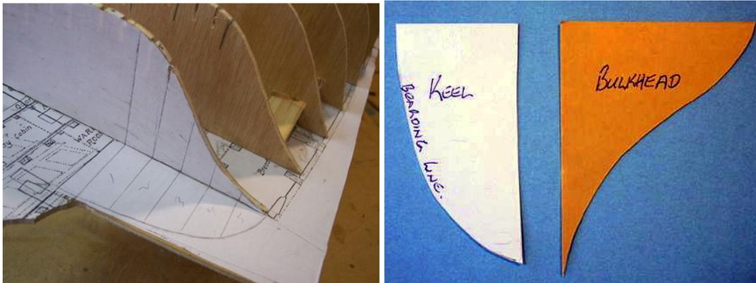
This time you need to measure the longest line on the bulkhead. In this case it was the uppermost filler block at position 1. This is going to establish the size of the block required. Do the same again on the keel. With these two measurements this is the size of the filler block for that segment. Do the same for all blocks using the longest line in all cases.
