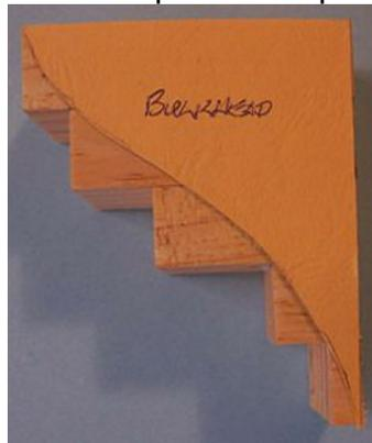
A template will need to be made up similar to the bow template from the keel plan using the bearding line as the final keel shape. Place this template on the keel side of the filler blocks and mark the shape.
