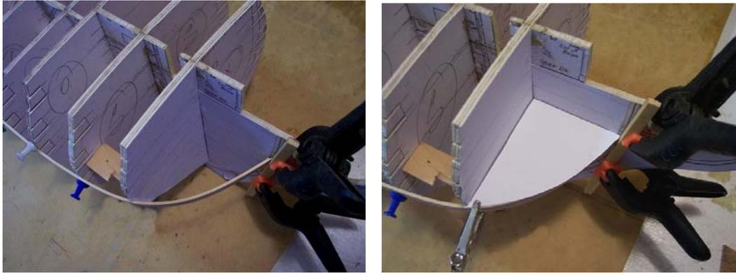
Cut the templates to shape leaving a fraction oversize to allow for final sanding. The blocks now look like an upside down wedding cake and still need sanding to final shape.
