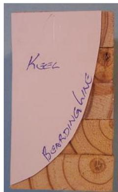
From your plans make up a template of the cabin floor or deck whatever the case may be. If you can't establish the final shape use a fairing strip to establish this shape if necessary using the same method as in the bow section.
