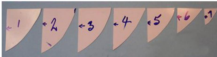
When the filler blocks are made up for both sides of the ship assemble them together BUT DO NOT GLUE them together at this stage. Take a pencil, and on the underside of each block draw the shape on the above block using the lower block as the guide. This line will show you the amount of material that has to be removed to establish the shape of that particular filler block.
